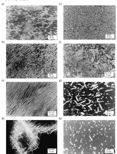
**Figure 2.**Textures evolution as a function of temperature for P<sub>11M</sub>/5CB mixtures (a) 27 °C; (b) 43 °C; (c) 55 °C; (d) 59 °C; and for P<sub>4M</sub>/5CB mixtures (e) 28 °C; (f) 32 °C; (g) 39 °C; (h) 48 °C.
